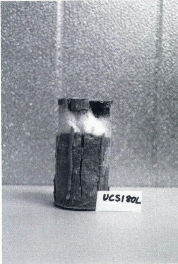
Fig. 6. A sample of laminated debris-laden basal ice after testing and failure at  $-25^{\circ}\text{C}$ . The sample failed suddenly by the development of an axial crack. The relatively clean ice layer towards the top of the sample is opaque as a result of microcracking.
