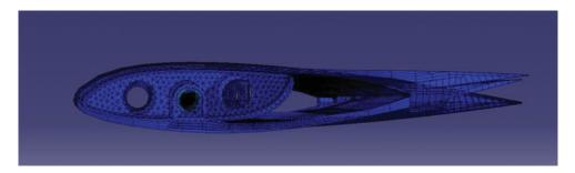
Figure 6. (Colour online) 3D deformed and un-deformed wing sections.
