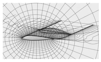
Figure 11. 3D mesh of the deformed wing in FP.
