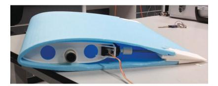
Figure 3. (Colour online) Morphing mechanism in situ in test section.
