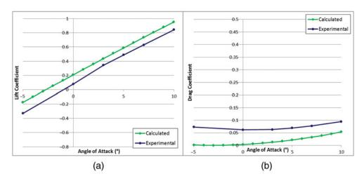
Figure 19. (Colour online) Lift (a) and drag (b) coefficient at 24 m/s; morphing activated.
