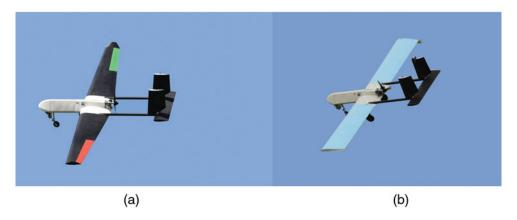
Figure 21. (Colour online) UAV Mark IV flying with conventional wings (a) and morphing wings (b).
