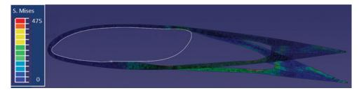
Figure 10. (Colour online) 3D deformed and un-deformed mesh of the Abaqus finite element analysis
