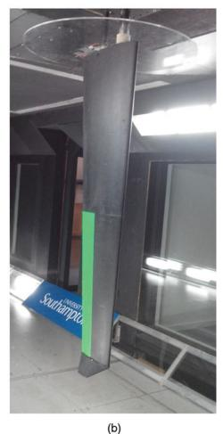
Figure 17. (Colour online) Wings in wind tunnel for test: morphing (a) and conventional (b).
