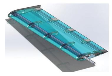
Figure 2. (Colour online) CAD model of the morphing wing – Note actuator on fourth rib.
