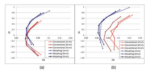
Figure 20. (Colour online) Experimental lift/drag coefficient comparison, un-activated (a), activated (b).
