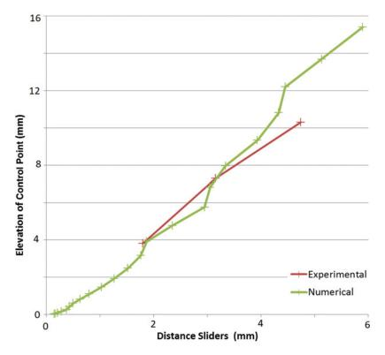
Figure 9. (Colour online) Comparison of computational and experimental deflections.
