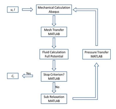
Figure 13. (Colour online) Aeroelastic analysis algorithm.
