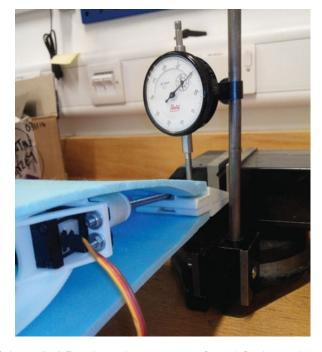
Figure 8. (Colour online) Experimental measurement of part deflection on short test section.
