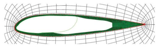
Figure 14. (Colour online) Abaqus and FP meshes superimposed.
