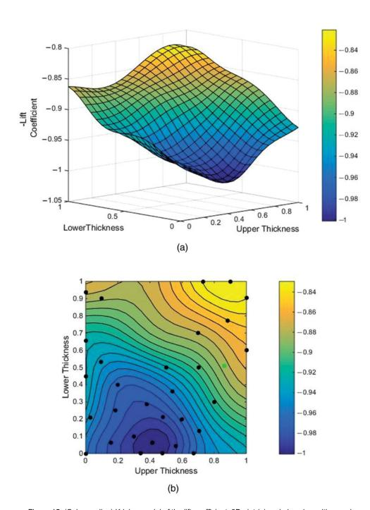
Figure 15. (Colour online) Kriging model of the lift coefficient: 3D plot (a) and plan view with sample points (b).
