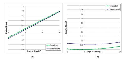
Figure 18. (Colour online) Lift (a) and drag (b) coefficient at 24 m/s; no morphing.
