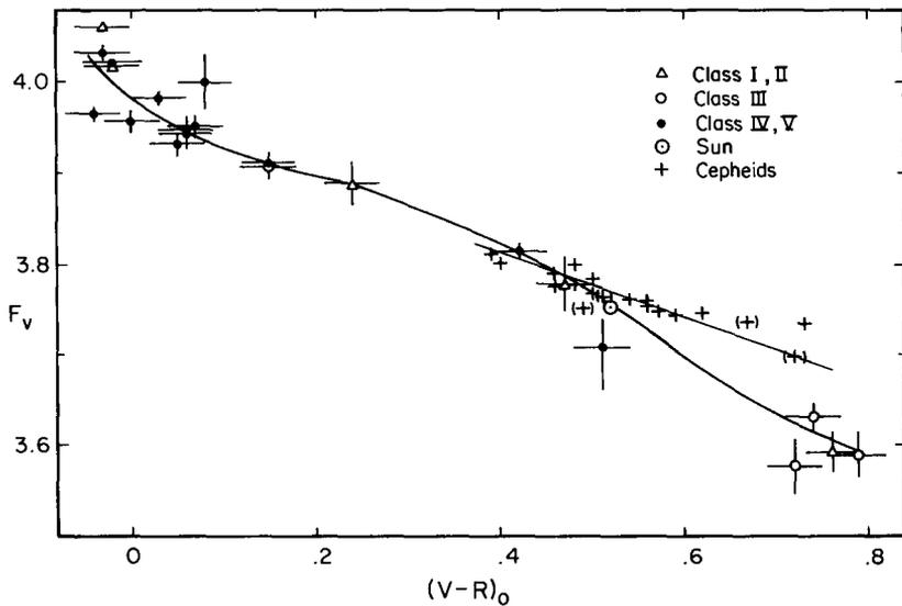
Figure 1: The relation between visual surface brightness parameter and  $(V-R)_0$  for Cepheids (plus signs) and for stars of measured angular diameter (all other symbols). Uncertain values are enclosed in parentheses.
