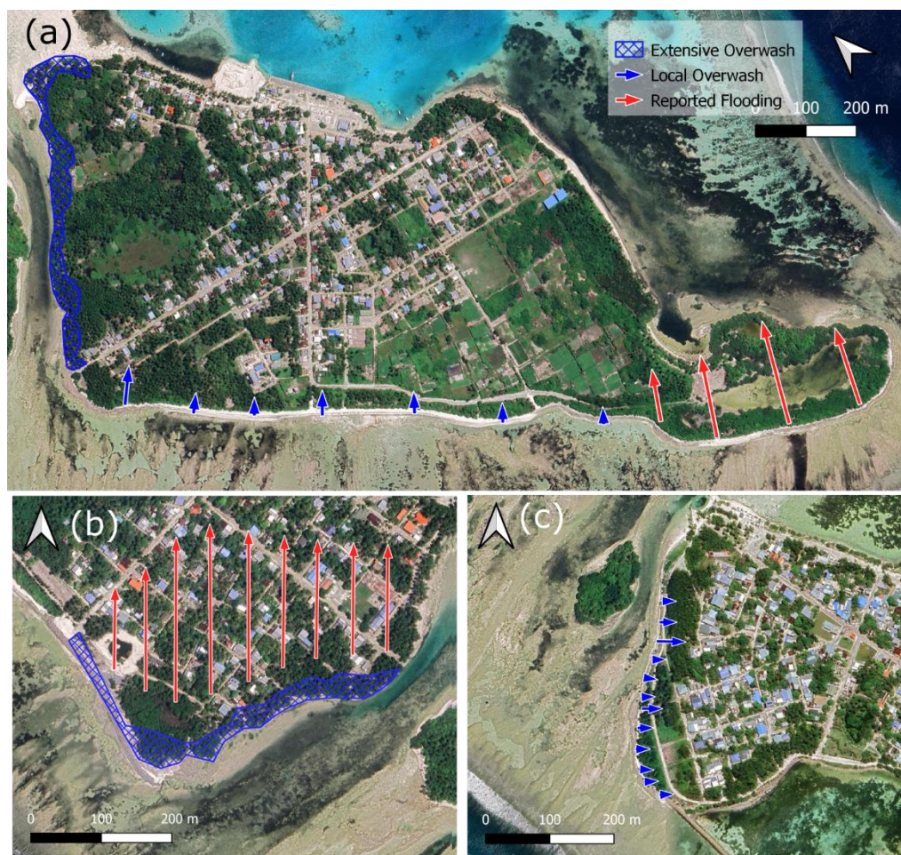
Figure 6 – Mapped extent of island flooding and overwash deposits recorded after 1 July flooding event: (a) Fioyaree; (b) SE margin of Rathafandhoo; and (c) SW margin of Fares-Mathooda. See Figure 1c for location of the three atoll islands. Source: GoogleMap.
