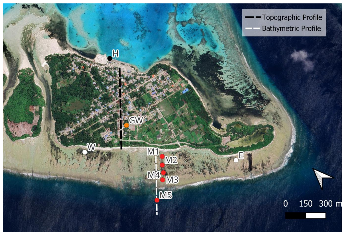
Figure 8 – (a) Satellite image of Fioyaree with location of all instruments during the July 2022 field campaign; and (b) assembled cross-island-platform profile derived from combined topographic (RTK-GNSS and electronic level) and bathymetric survey (single-beam echosounder) with the locations of the wave sensors on the central transect. Source of (a): GoogleMap.
