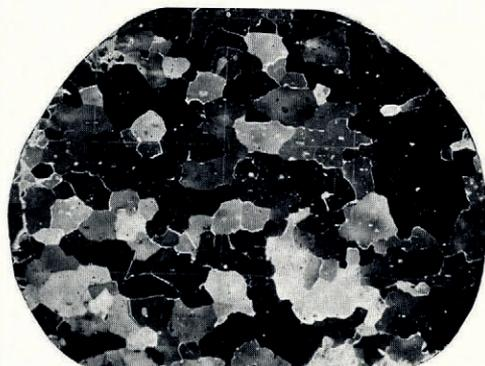
Fig. 2. One of the serial thin sections used in tracing crystals. Crossed polaroids. Grid spacing 20 mm. Section diameter about 70 mm.
