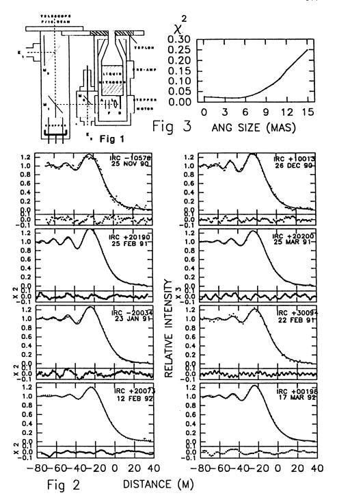
corresponding to 26 arc sec on the sky at the 1.2 m telescope, whenever the photometer is used in the slow (photometry) mode. In the fast (occultation) mode there is no sky chopping and the detector/preamplifier output is directly digitized with a 16 bit A/D converter and recorded in a PC based data acquisition system. Data sampling is at the rate of 1 millisecond for 30 seconds centred on the predicted time of the occultation event.
