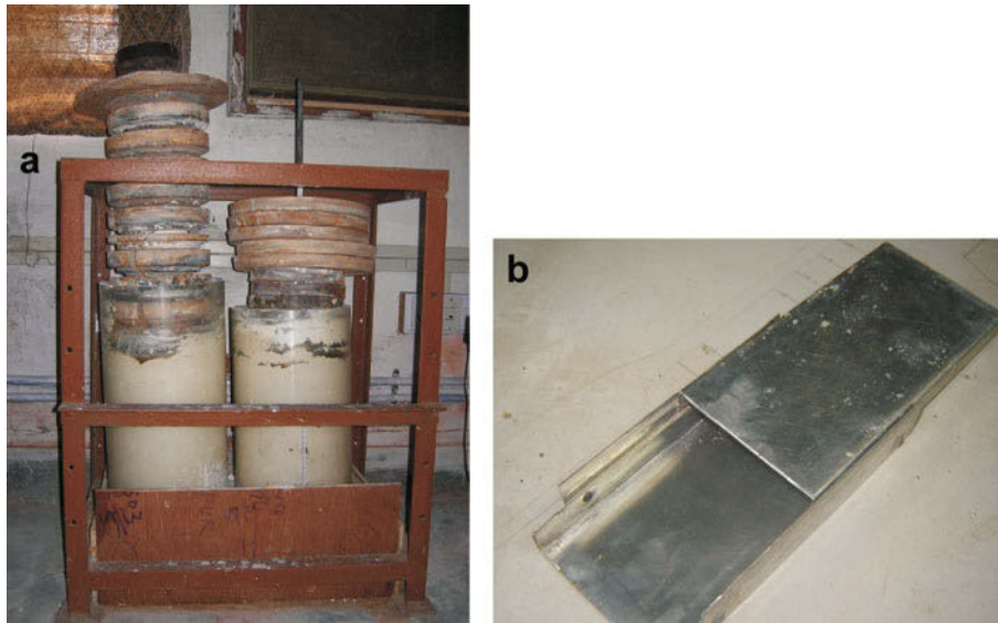
Figure 2. (a) Slurry (or consolidation) tank (450 mm in diameter). The vertical consolidation loads are visible at the top of the perspex tanks. The sand bath is not visible; (b) rectangular split mold (150 mm long, 75 mm wide, and 30 mm thick).
