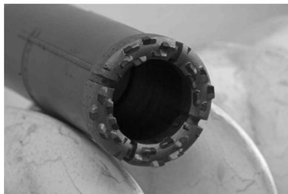
**Fig. 5.** Temperature-stabilized diamond rock-coring bit.
