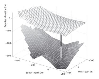
**Fig. 5.** Oblique view of the study site. Upper and lower surfaces show the glacier surface and bed, respectively. The grid size of the mesh is  $20 \text{ m} \times 20 \text{ m}$ . The vertical column indicates the drilling site, with dark gray representing the retrieved 180.17 m long ice core.
