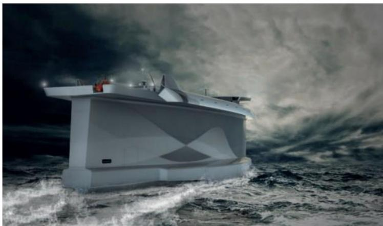
Inspired by airfoil techniques harnessed by the aviation and sailboat industries, Vindskip's wind-powered propulsion enables a 63% reduction in CO<sub>2</sub>
