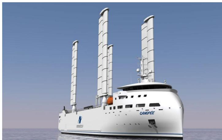
Figure 6: Example of ship equipped with hard sails
