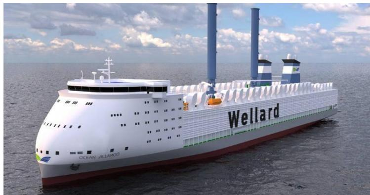
Figure 5: Flettner rotors fitted on a ship's weather deck
