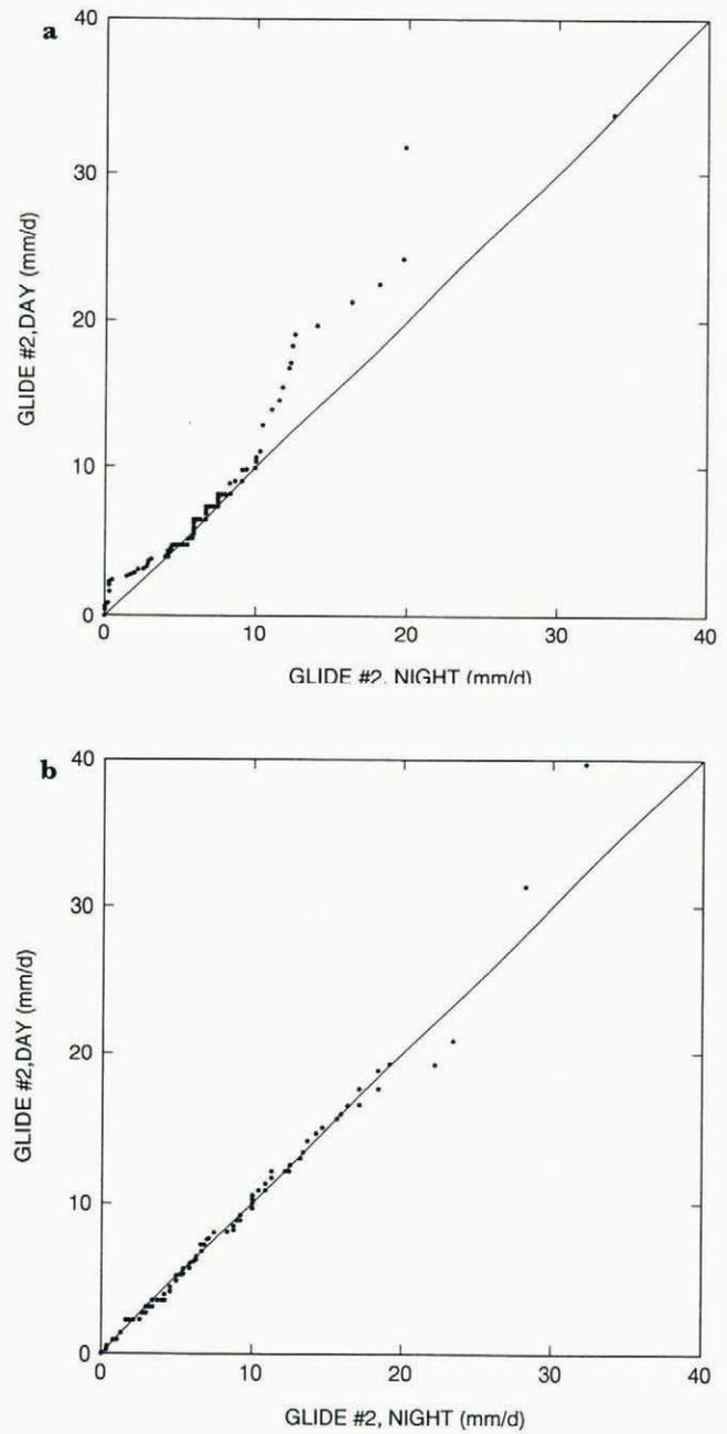
Fig. 5. Quantile-quantile plots of glide rates for day (0600–1800 h) versus night (1800–0600 h) at gauge #2. a, 1988–89 winter. b, 1989–90 winter. Note: glide rates are plotted as  $\text{mm d}^{-1}$  (24 h period).
