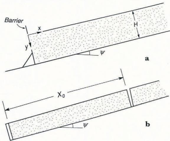
Fig. 6. Schematic for calculation of stresses on a barrier on a slope subject to snow gliding and slip. a, Equation (3) gives the longitudinal stress on the barrier for moderate gliding without presence of a tensile crack. b, Equation (6) gives a simple formulation for rapid sliding (zero friction) when a tensile crack forms upslope from the barrier.
