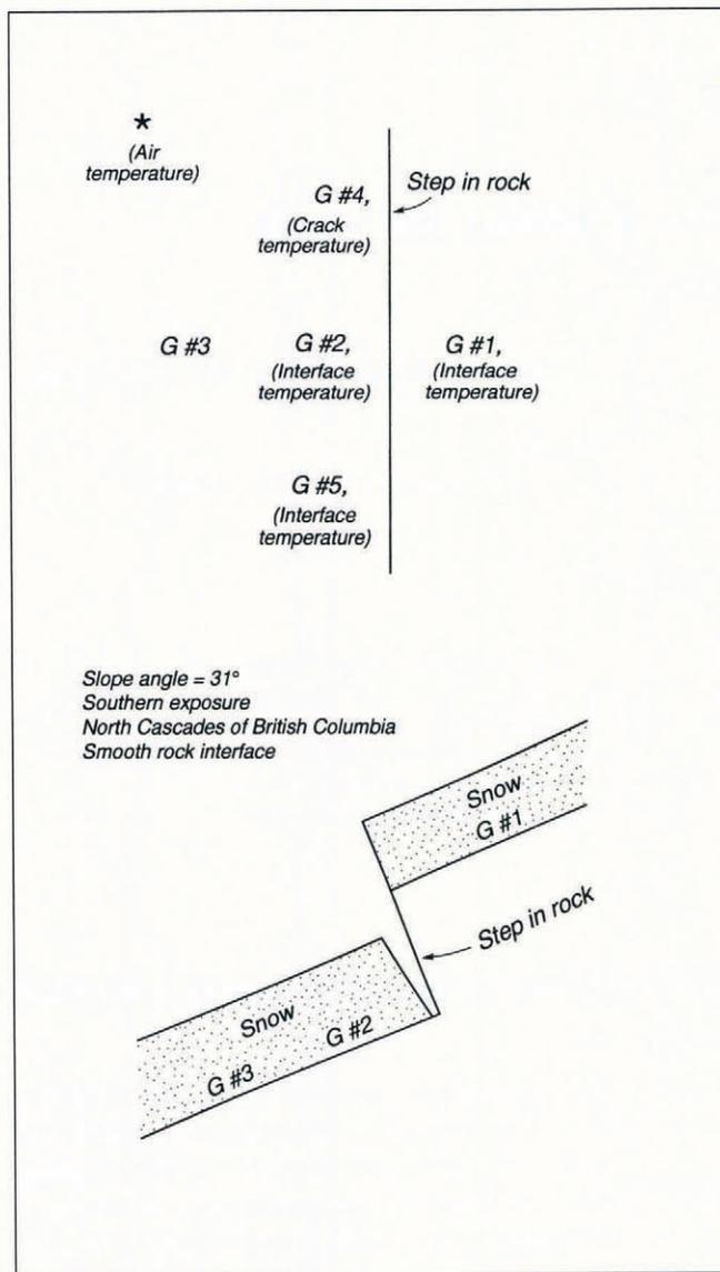
Fig. 1. Plan and side views of snow glide gauge placements (G#1 through G#5) relative to a 2 m high step in the rock. Glide interface temperature measurements are made at G#1, G#2 and G#5. Also shown are locations of thermistors in the glide crack between the step in the rock and the snowpack and air temperature 3 m above the snowpack. A side view shows the configuration of the rock and snowcover.
