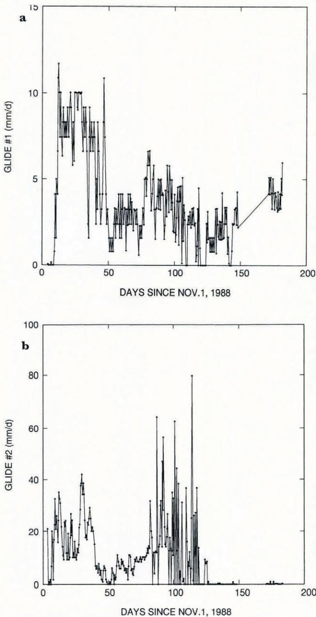
Fig. 3. Glide speed ( $\text{mm d}^{-1}$ ) measurements based on two 12 h averages (0600–1800 h; 1800–0600 h) per 24 h periods (1988–89 winter). a, Gauge #1. b, Gauge #2. The gauge exceeded the displacement limit past day 130.
