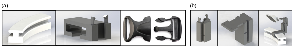
Figure 4. CAD model showing: (a) Guide rail base, Sleeve with compliant mechanisms and compliant snap-fit buckle, (b) Horizontal Rail and Final assembly
