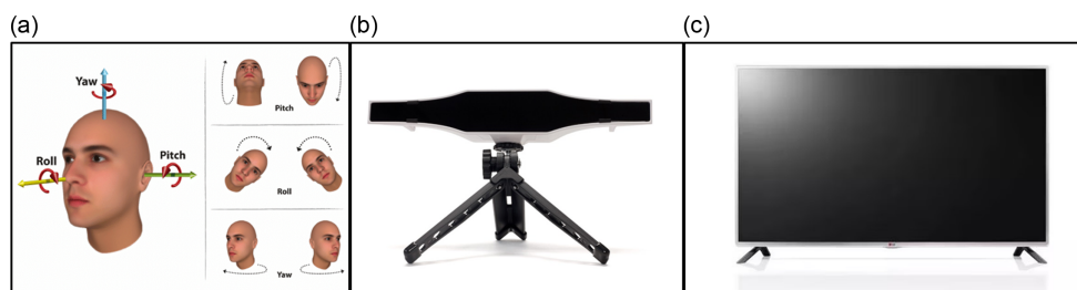
Figure 1. (a) Head yaw, roll and pitch movements significantly affect eye-trackers' accuracy in larger screens (Rozali et al., 2022), (b) Gazepoint GP3 HD eye-tracker, and (c) LG 47-inch LED HDTV used for testing
