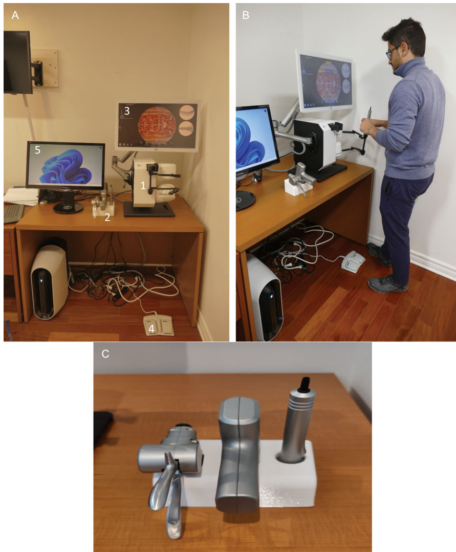
Figure 1. TSYM virtual reality simulator platform developed by Cedarome Canada Inc. dba Symgery (Montreal, Canada) (A) The TSYM simulator set up, showing the (1) robotic arm that uses and provides advanced haptic feedback technology, (2) the different tool handles that can be used in the simulated scenario, (3) 3D monitor, (4) pedals for activating fluoroscopy and (5) secondary monitor. (B) A neurosurgical resident performing a task on the simulator, demonstrating its practical use in a training scenario. (C) The tool handles are available to mimic an array of tools in the virtual environment.
