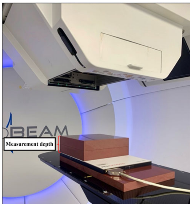
Figure 2. The patient-specific QA setup for each plan.
