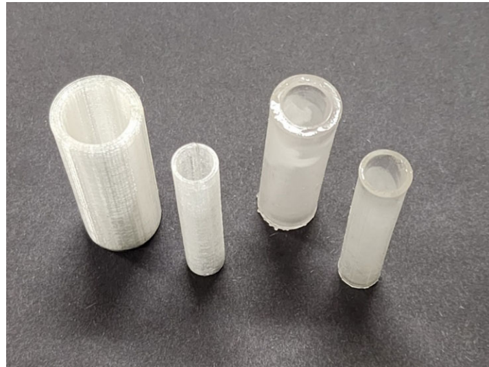
Figure 6. Fabricated tubules for TPU (left) and SLA parts (right)
