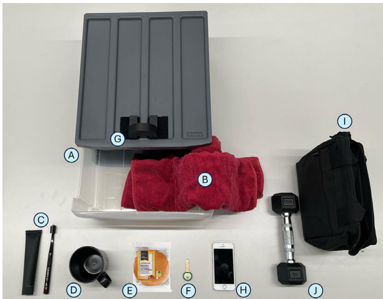
Figure 4. Materials for the ADL tasks. On top: a drawer (A) with a red towel (B). On the bottom from left to right: a toothbrush and toothpaste (C), a black cup (D), a packaged Biberli (E), a key (F) (3D-printed keyhole on top of the drawer, G), a smartphone (H), and a black bag (I) with 1 kg weight (J). The weight inside the bag during testing.
