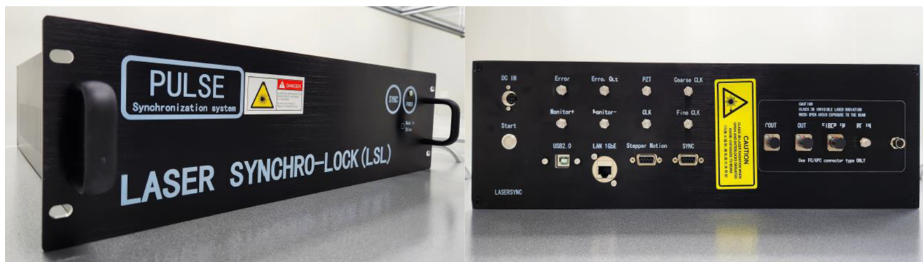
Figure 12. Laser-to-laser synchronization module in SHINE.
