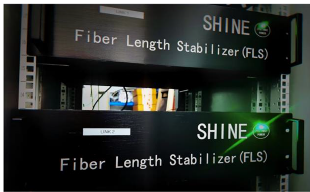
Figure 7. Fiber length stabilizer at SHINE.
